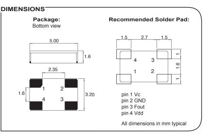
SMT Voltage control oscillator in ceramic package Fundamental quartz mode frequency High shock and vibration resistance Wide temperature range Low aging Ultra low internal MSL Very fast start-up Excellent solderability Swiss made quality Customer specification on request
