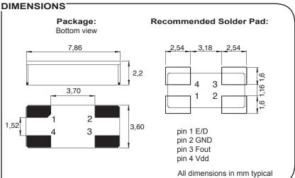
SC cut quartz crystal SMT Clock oscillator in ceramic package Fundamental quartz mode frequency Ultra Low stability High shock and vibration resistance Wide temperature range Low aging Ultra low internal MSL Very fast start-up Excellent solderability Swiss made quality Customer specification on request
