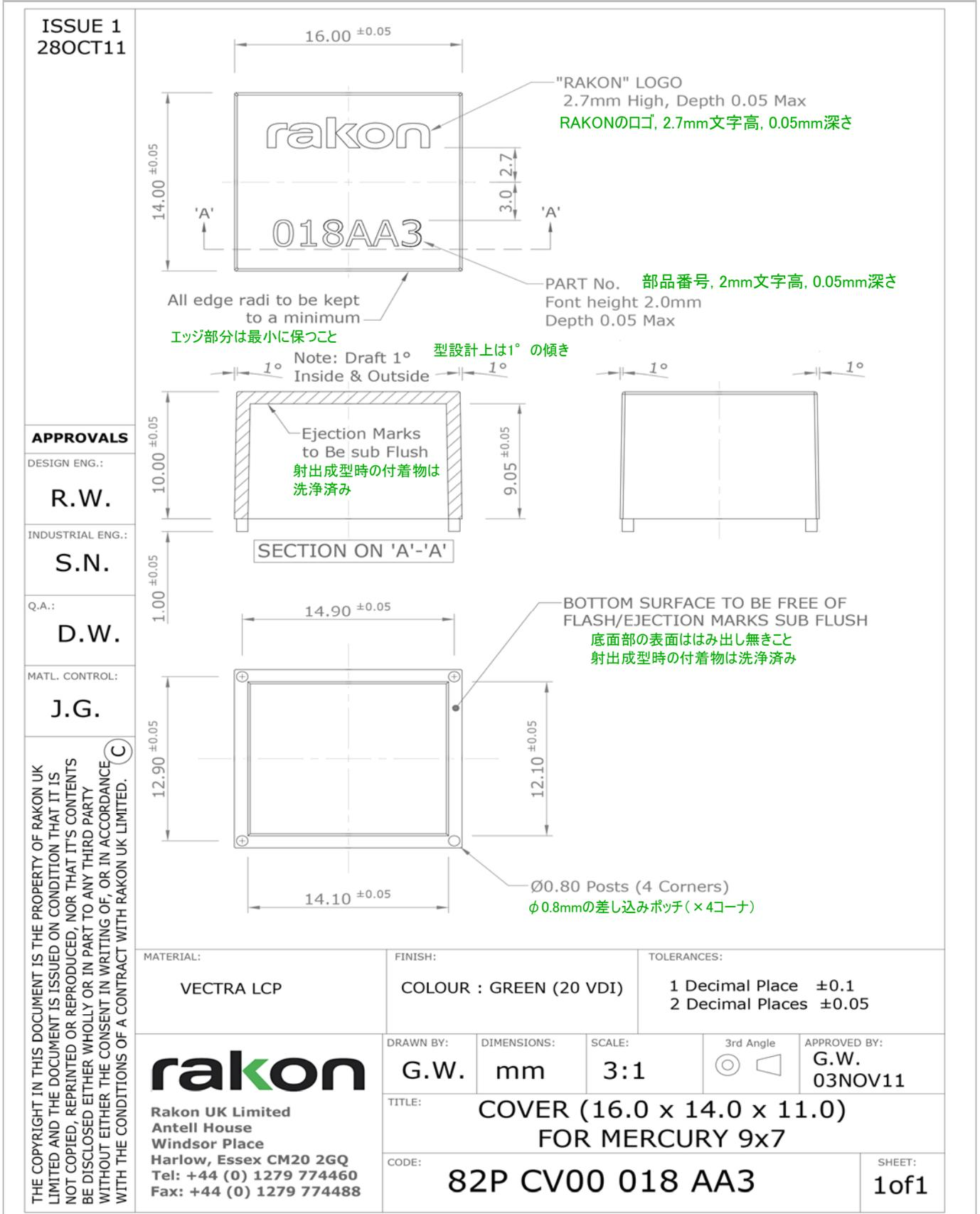
Figure 5: RFPO40 / RFPO45 Model and Cover Assembly
